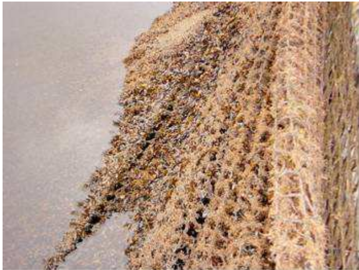
A net covered in a variety of organisms that can affect the flow of water through the net
