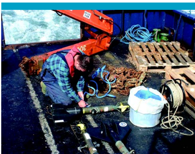
Deployment of self recording current meters for hydrographic measurement.
