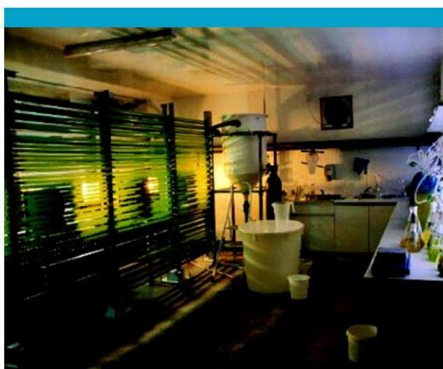
Continuous algal production system in the algal room at the new Machrihanish Marine Farm Ltd cod hatchery.
